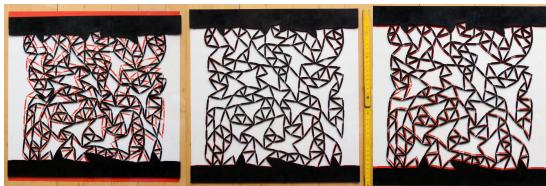
Figure 1: Experiment with laser-cut auxetic network. Compression (left) and extension (right) of a laser-cut auxetic irregular network in rest state (middle) computed by our purely geometric process. Notice the horizontal, transversal contraction (left) and extension (right) characteristic of an auxetic behavior. The compressed network exhibits a Poisson's ratio \nu = -0.94 for an applied strain \varepsilon_y = -7.1\% . The extended network exhibits a Poisson's ratio \nu = -0.46 for an applied strain \varepsilon_y = +3.3\% . Strains are applied symmetrically to the top and bottom boundaries.
